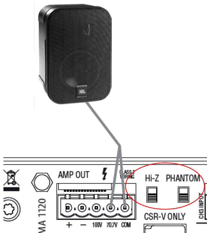
**Note:** Wire to appropriate terminals for configured output mode. 70volt mode shown in figure above.
